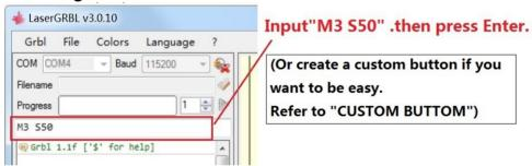
The laser will be turned on with low power model. Then Rotate the lens to minimize the spot.
